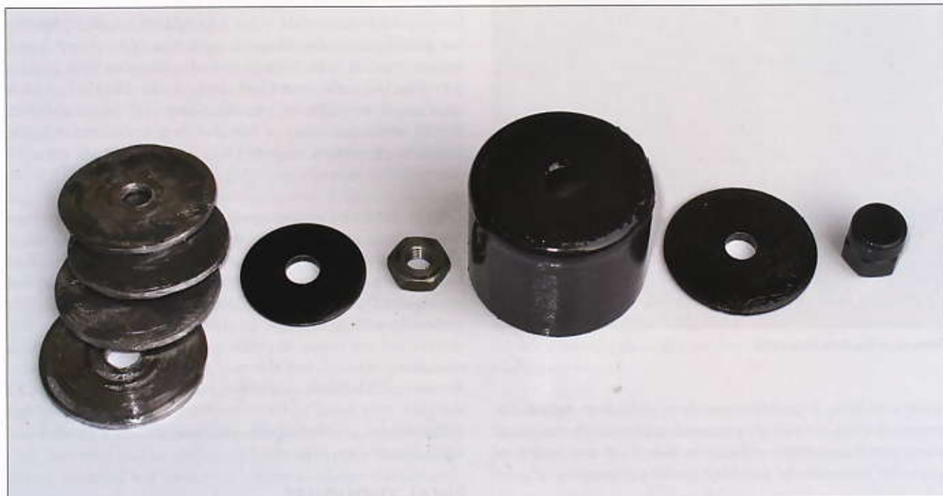
Correct assembly order of the lead weighting discs (variable number as required), conical washers and 'cotton reel' cover. Three of these assemblies are fitted to each road wheel.
