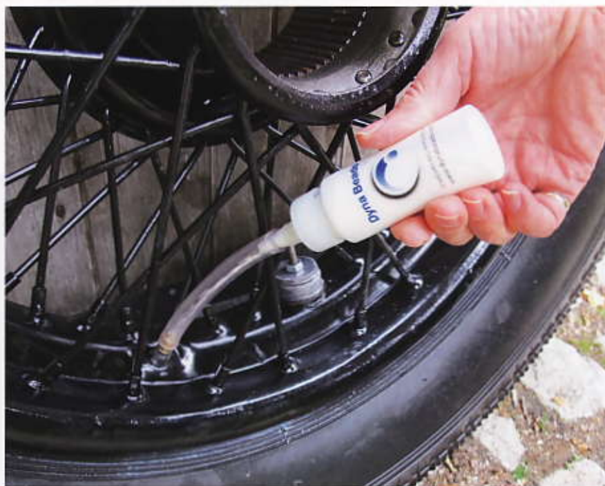
Ceramic beads being injected using an applicator.
